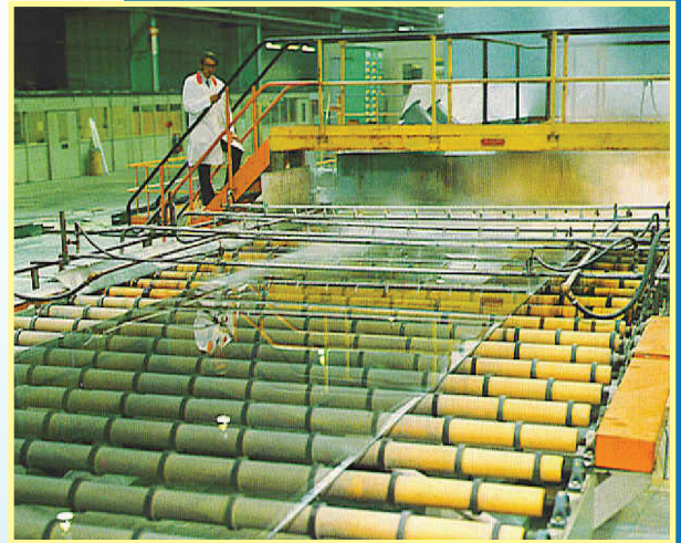
A long, flat layer of cooled glass comes out of the lehr to be washed and cut.
